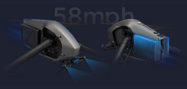
Structure: Magnesium aluminium composite shell and transforming design, carbon fiber arms
