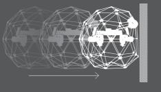
With a spherical cage protecting propellers from impacts, Elios 2 remains always stable through lightning-fast corrections on the propellers' speed and direction of rotation. The entire payload is mounted on a retractable structure that protects it from damages in case of frontal shocks.
