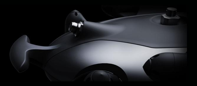
The E-GO's biomimetic tail fin is derived from a nature-inspired design, offering multiple functionalities. It stabilizes the drone during underwater operations, minimizing water flow disturbances.
